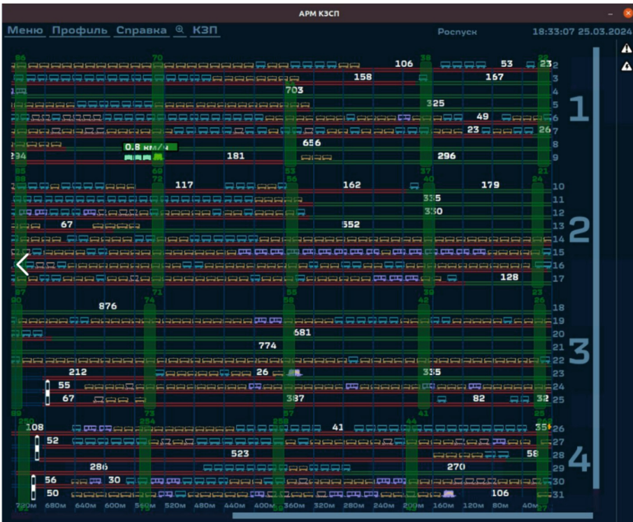
Fig. 2. Screenshot of the longitudinal profile analysis working window at WS KZSP (Profile designation colors: red – accelerating slope, green – slope within normal limits, yellow – decelerating slope).
